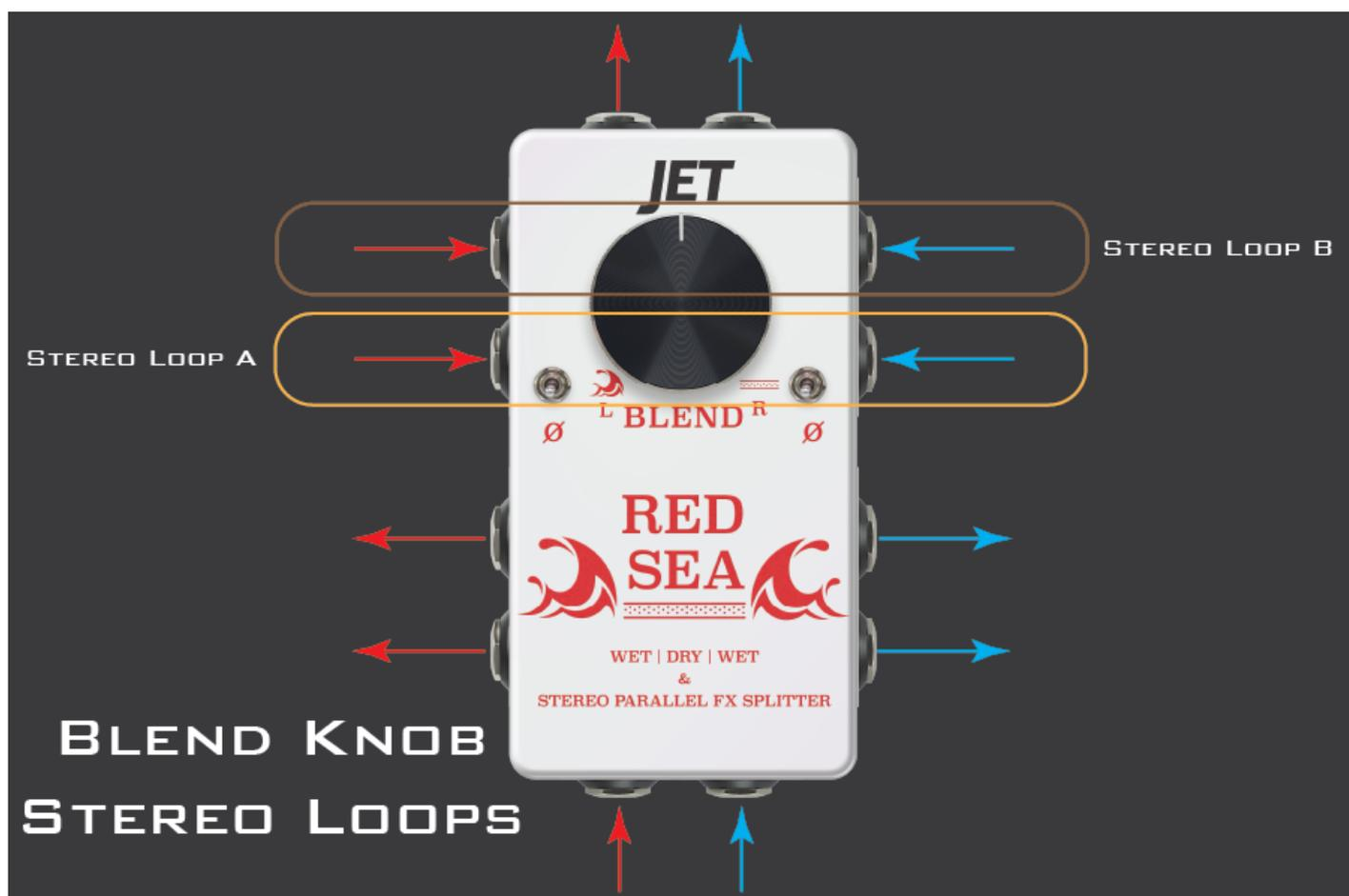
It can also be used to blend the overall mix between your dry and wet signals when using the Red Sea for Wet Dry Wet. When rotating the Blend knob counter clockwise, the Wet loop (Return Jacks 1 & 3) will get louder while simultaneously making the Dry loop (Return Jack 2) quieter. The opposite is true when rotating the Blend knob clockwise, Dry gets louder while Wet simultaneously gets quieter.
