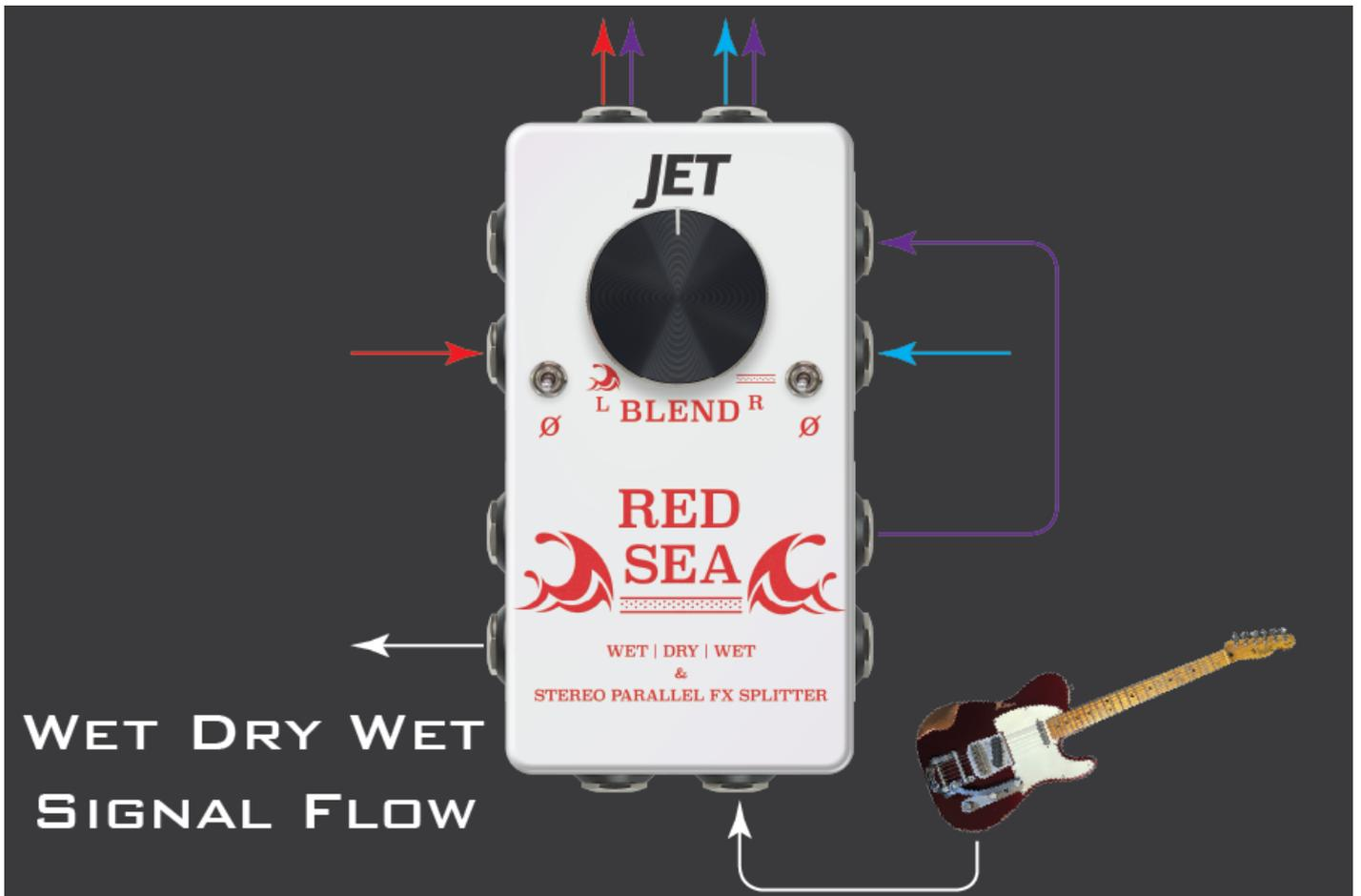
Hopefully by now you can see how your signal will flow in and out of the Red Sea. Later in the manual we will provide various wiring diagrams for different routing options, however using the knowledge above you should be able to create your own unique routing configurations.
