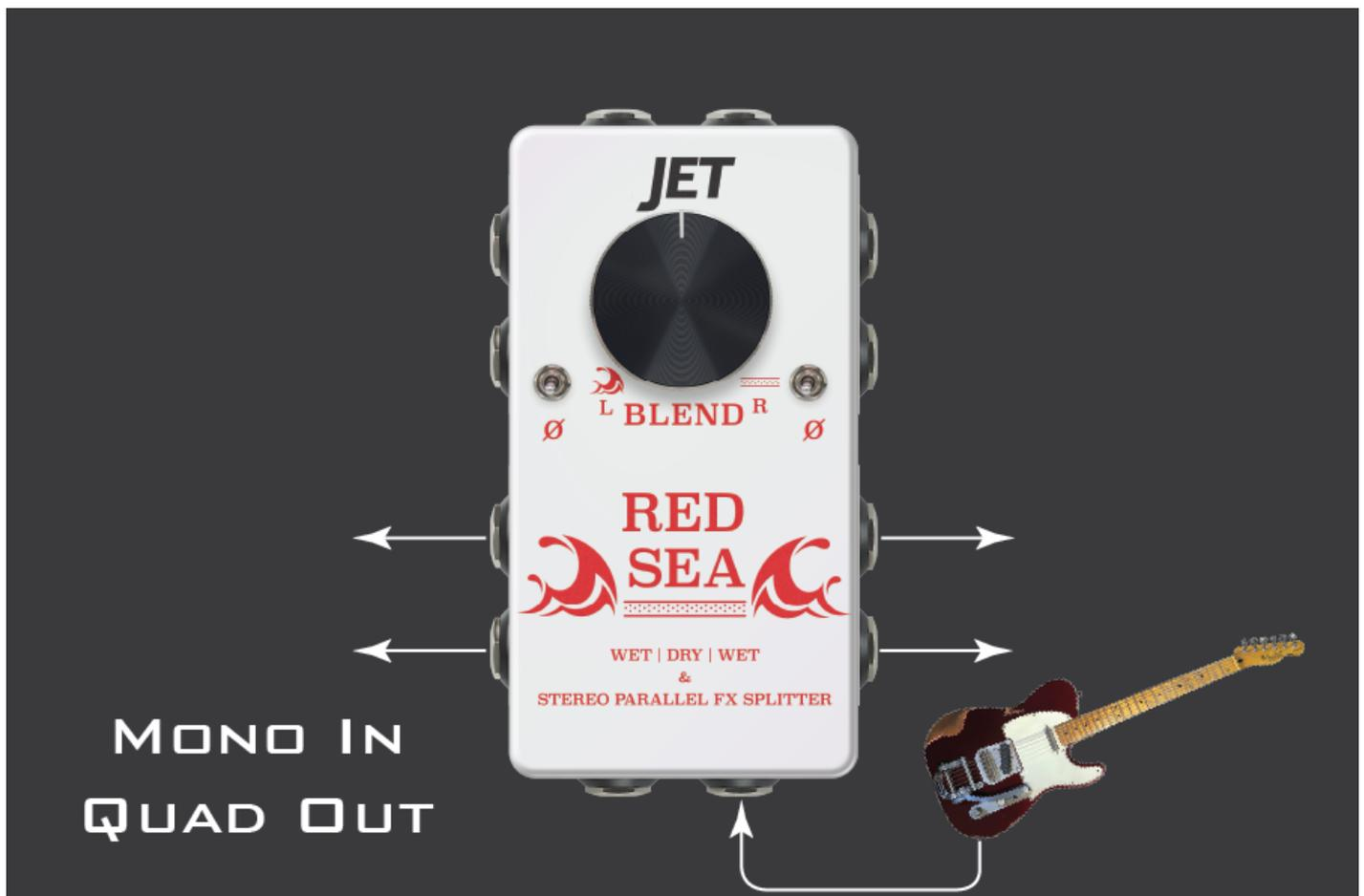
Use both Left and Right inputs to maintain a stereo image routing through the Red Sea. When ran in stereo, the Left Input will be copied, split, and sent to send jacks 3 and 4. The Right Input will be copied, split, and sent to send jacks 1 and 2. The input signals can be anything like dual guitars, 1 guitar and 1 bass, or any stereo effects pedal.
