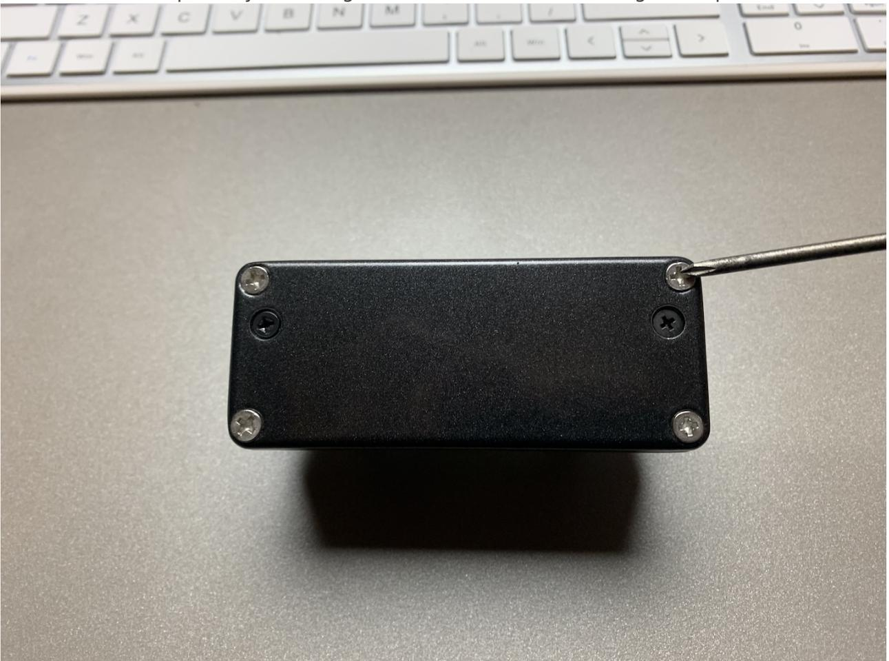
2. Remove the backplate from the PCB by removing the two black screws.
