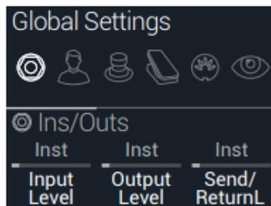
3. Turn the Upper Knob to select one of the six submenus. If necessary, press PAGE ▶ to view more parameters.
